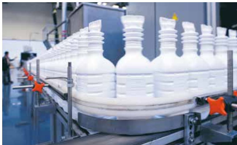
Left: injection moulding. Right: extrusion-blow-moulded bottles on the way to the next processing step.
